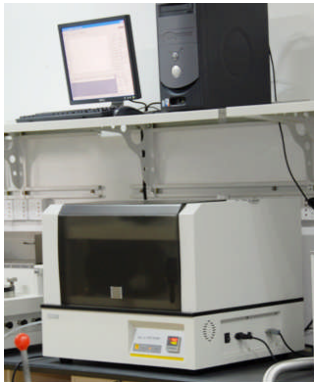
Figure 2. VAC-V1 Differential Pressure Method Gas Permeability Tester
