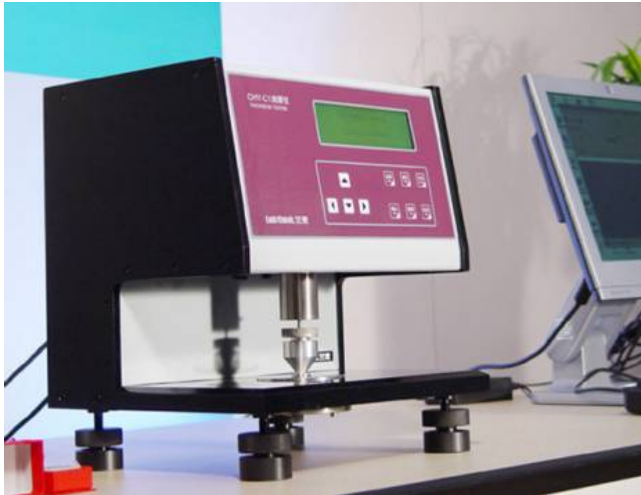
Fig.1 Labthink CHY-C1 Thickness Tester
