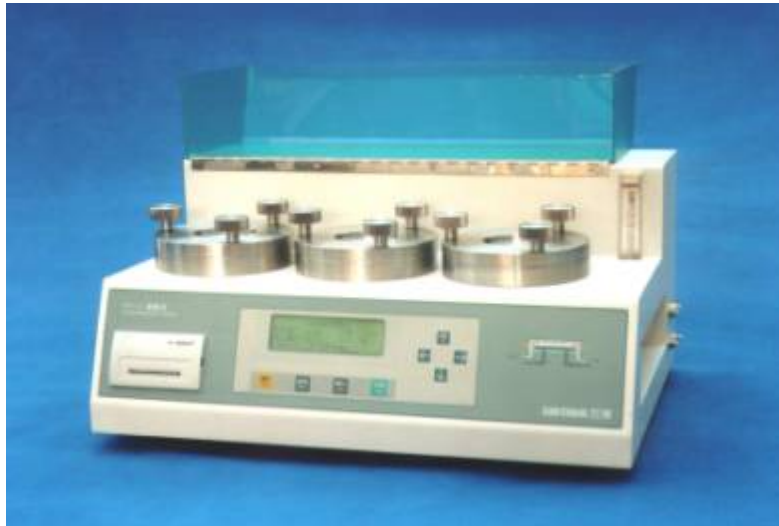
Fig.3. TOY-C1Package/Film Oxygen Permeability Tester which has fitted with the sample in film type
